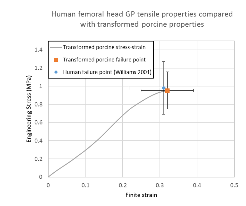
Figure 6-11: The transferred porcine engineering stress-finite strain curve using the correlation factor X_{opt} . The estimated failure point for 10 YO was plotted together with the that from human GP tests (William et al., 2001). The ranges of stress and strain with plus/minus one standard deviation were given
